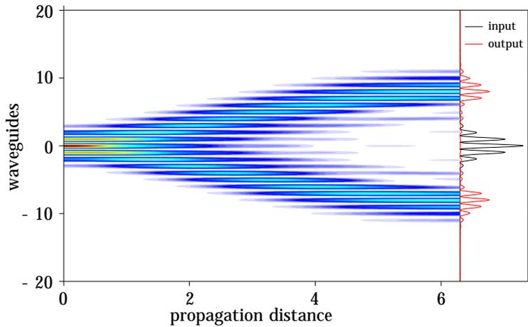
FIG. 3. (Color online) A Gaussian beam splits during propagation in a V-type modulated waveguide arrays. The 0 waveguide is excited by the beam peak. Curves in the right panel are the corresponding beam intensities at input and output places, respectively.
