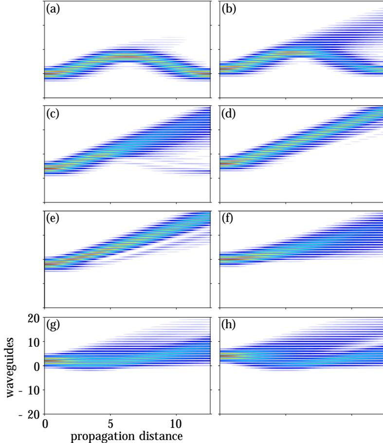
FIG. 2. (Color online) Propagation of the light beam in periodic waveguide arrays with  $\alpha = 0.5$  for  $m \leq 0$  and  $\alpha = 0$  for  $m > 0$ . (a)-(h) Peaks of the incident beams locate at the waveguides  $-10$ ,  $-8$ ,  $-6$ ,  $-4$ ,  $-2$ ,  $0$ ,  $2$ , and  $4$ , respectively.
