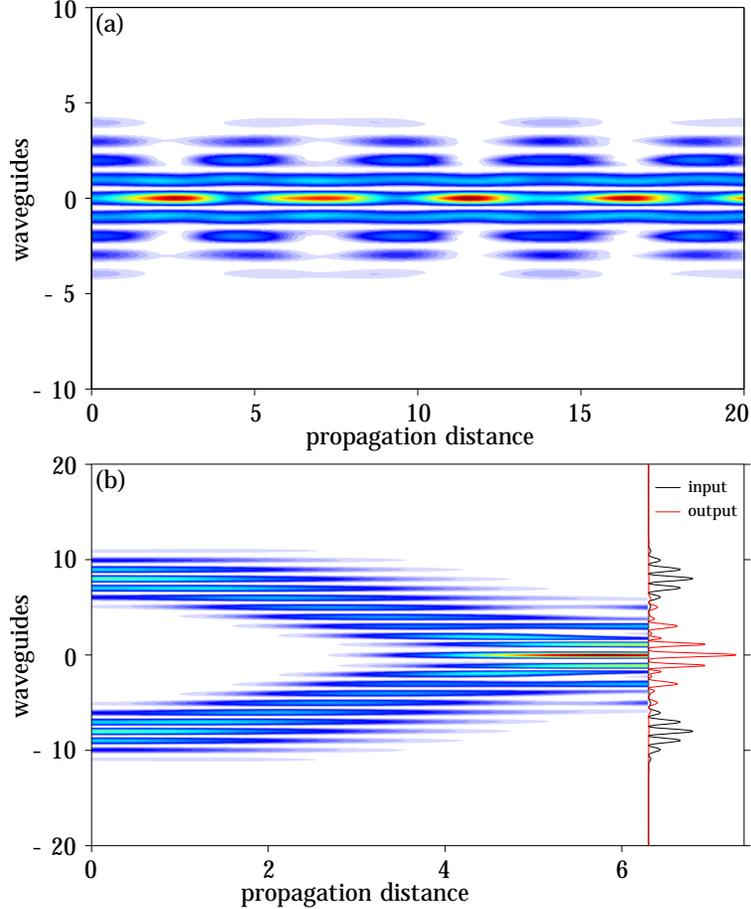
FIG. 4. (Color online) (a) Propagation of a Gaussian beam in the  $\Lambda$ -type modulated waveguide arrays with the 0 waveguide excited by the beam peak. A Fermi-Pasta-Ulam recurrence-like localization happens during propagation. (b) Two Gaussian beams respectively launched from positive and negative waveguides coalesce during propagation. Curves in the right panel are the corresponding beam intensities at input and output places, respectively.
